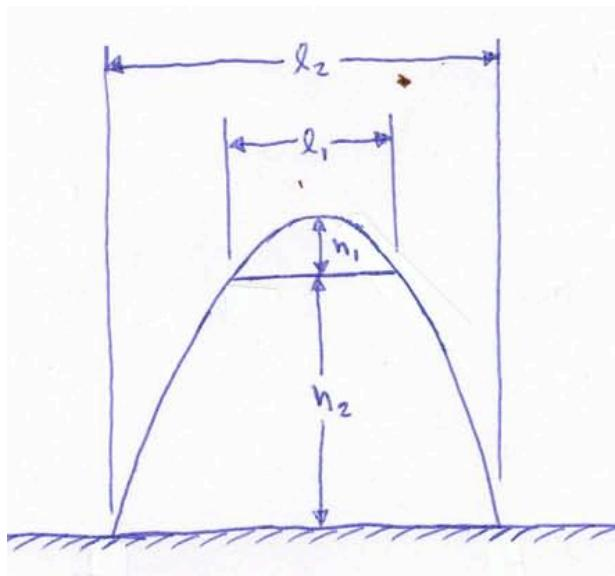
(5 marks) A hydro wire hanging between two poles could be expressed with a 2nd order polynomial. If the hydro poles are 50m apart and the maximum sage in the wire is 2m, determine the equation of the wire between the two poles.
