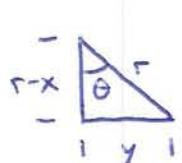
$$y = \sqrt{r^2 - (r-x)^2} \Rightarrow \text{Area} = \frac{(\text{base})(\text{height})}{2} = \frac{(r-x)[r^2 - (r-x)^2]^{\frac{1}{2}}}{2}$$
