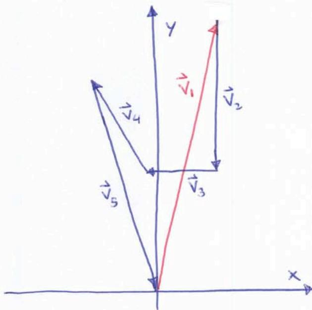
$$\vec{V}_1 + \vec{V}_2 + \vec{V}_3 + \vec{V}_4 + \vec{V}_5 = \vec{V}_f = 0$$
